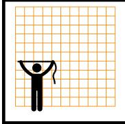
Determine the position of the first a horizontal line to serve as the start of the panel arrangement.
