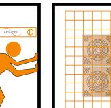
Place, level and hold the panel against the wall for at least 2 minutes while the glue straightens.
